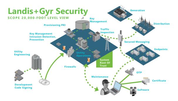
Landis+Gyr's Gridstream Connect solution provides utilities with a highly flexible, interoperable, open
