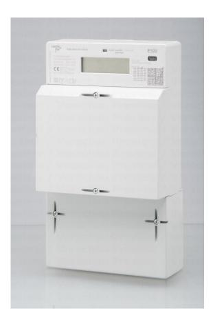
The E320 FNN base meter meets all the requirements set by the Digitisation Act and the FNN. It fits both 3-phase 4-wire and 1-phase 2-wire applications. The E320 is an SLP meter that also delivers GRID values at the LMN interface. Optionally, it may be parameterised to deliver additional RLM values.
