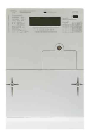
The E220 standalone meter meets all the requirements set by the Digitisation Act. It is designed to meet most of the FNN requirements for base meters and suits both 3-phase 4-wire and 1-phase 2-wire applications. The E220 is an SLP meter that also delivers GRID values. Optional modules available include a Dual Tariff Module or an LMN interface (alternatively RS-485 or wireless M-Bus).
