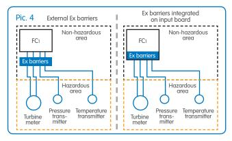
The ExMFE5 input board has integrated barriers (picture 4 right hand side). The advantage of this board is that the transmitters and e.g. the turbine meters can be connected directly to the board without any peripheral devices. This saves costs and space within the cabinet.
