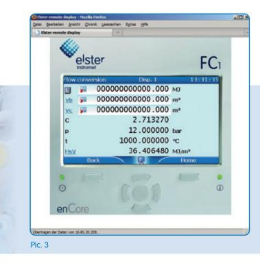
It is used for parameterization purposes archive readouts and SCADA communication. An http:// web server is implemented with which a remote operation panel can be transmitted all over the world (picture 3) for maintenance reasons.
